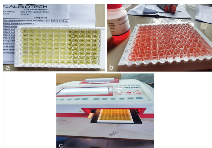
[Table/Fig-1]: a) Showing diluted specimens and diluted controls were dispensed into appropriate wells; b) Showing enzyme conjugate reagent was dispensed into each well; c) Absorbance was noted at 450 nm with a microtiter well reader.
