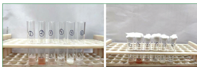
[Table/Fig-1]: Sets of fluids examined were prepared in two test tube racks one containing fluid plus alcohol mixture left to stand at room temperature (a); and another set of test tubes with alcohol plus sample was kept in the fridge (b). (Images from left to right)
