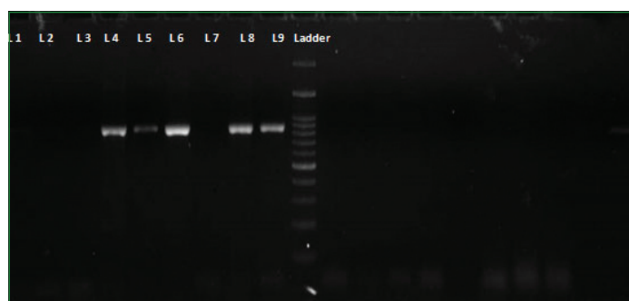
[Table/Fig-1]: Agarose gel electrophoresis showing amplicons of VP7 gene and VP4 gene. Amplicons of base pair size 881 in lane 4, 5 and 6 are of VP7. Amplicons of VP4 gene (876bp) are seen in lane 8 and 9. A 100 base pair molecular marker is run in lane 10. Lane 6 and 9 are of control strain Wa-1.
